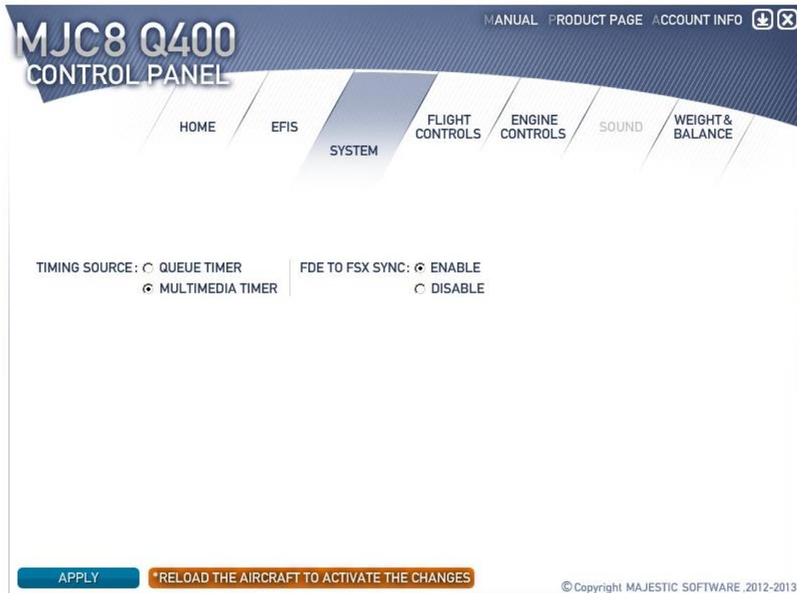
The MJC8Q400 addon has a complex multithreading infrastructure, with different threads running with its own rates, to make the best use of the multiple processing cores. There are numerous additional settings available directly in the mjc84.ini file, and the 2 most important of them are configurable in CPAN:
